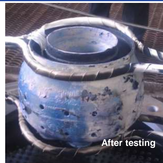
CMC liner testing
